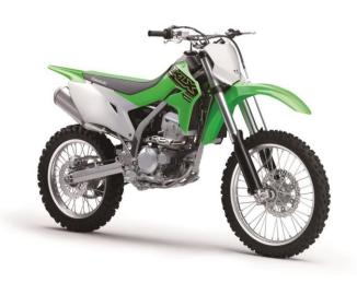
wheels and tires, using a 21" front and 18" rear, and long travel suspension for optimal ground clearance.
