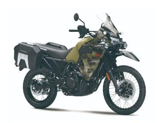
that rides on a recently redesigned high-tensile double-cradle frame. Its LED headlight, all-digital multifunction instrumentation, optional ABS system, and 7.9" of front travel coupled with 7.3" of rear travel ensure that it's ready to go for any journey on- and off-road.
