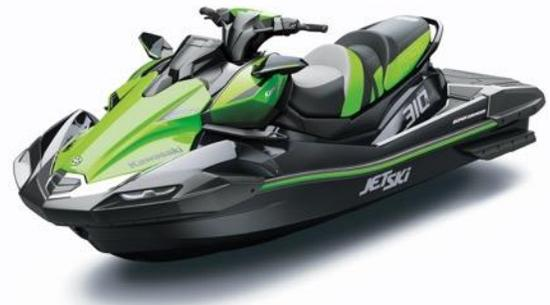
Developed for fun, excitement, and comfort, the Jet Ski Ultra 310 series is powered by the legendary liquid-cooled, supercharged, in-line 4-cylinder, 1498cc marine engine and when paired with new features including launch control, power mode selection, and an array of equipment features, the Jet Ski® Ultra® 310X leaves little to question. For 2022, the Ultra 310 line will come in three model variations with the Jet Ski Ultra 310X, Jet Ski® Ultra® 310LX-S, and the Jet Ski® Ultra® 310LX.
