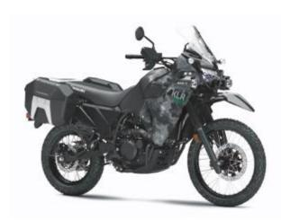
The all-new 2022 KLR650 receives the addition of fuel injection to the 652cc single-cylinder engine
