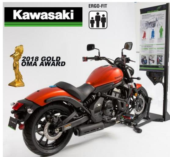
The ERGO-FIT system features a combination of adjustable components for riders of different stature to help fit the motorcycle to the rider. Developed and constructed by One Source Industries (OSI) the ERGO-FIT display allows riders to sit on a Vulcan S motorcycle and try the different positions in handle bar and foot peg positions as well as multiple seats while taking up very little space on a dealer's showroom floor.
