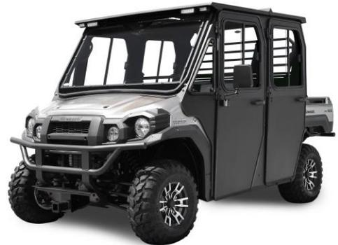
The Curtis cabs are made in the USA and feature a total weather seal design, a venting hardened polycarbonate or glass windshield and safety glass door sliders that can be removed quickly to increase airflow. They also come with gas-shock supported lockable doors that provide smooth opening, an acoustic headliner, and a wide range of optional accessories.
