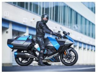
the machine is a hydrogen engine based on the 998 cc In-Line Four Supercharged Engine found in Kawasaki's Ninja H2® motorcycle, with modifications made to allow direct injection of hydrogen fuel into the cylinders. The motorcycle's chassis was designed to accommodate hydrogen fuel canisters and a hydrogen fuel supply system on-board.
